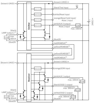
01) This wiring is used to activated the lamp output and displays the status to the external indicator based on 02) RS485(A) and RS485(B) are for the synchronous line.
