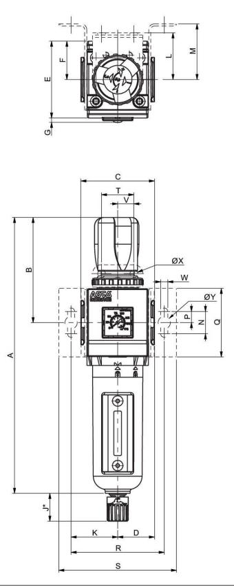
To remove the reservoir, allow a clearance of [[80] mm] from the bottom of the reservoir drain. \*Variable dimension based on the type of drain specified, if an automatic drain is specified, add another [[5] mm] to the "J" dimension.
