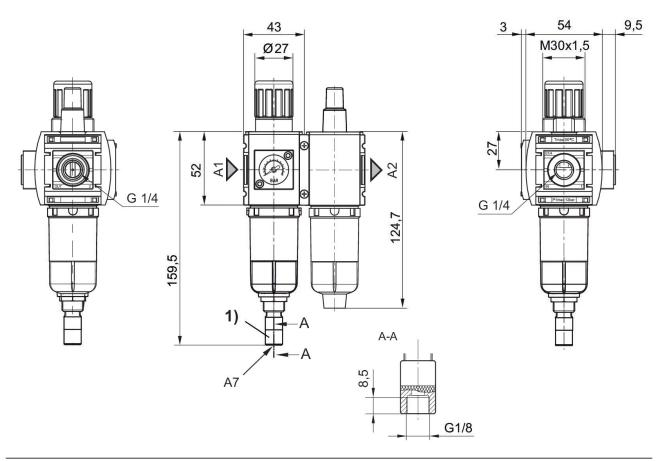
A1 = input A2 = output A7 = condensate drain 1) Fully automatic condensate drain
