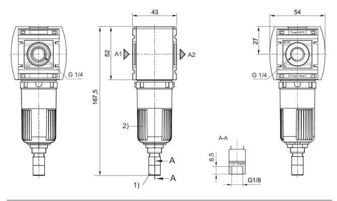
Fully automatic condensate drain
