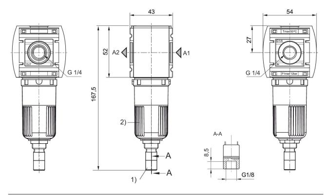
Fully automatic condensate drain Reservoir: polycarbonate
