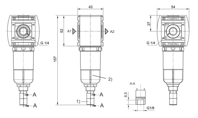
Fully automatic condensate drain
