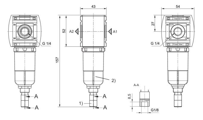
Fully automatic condensate drain
