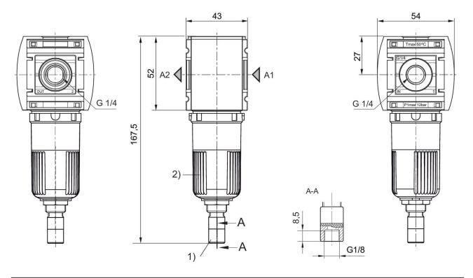
Fully automatic condensate drain
