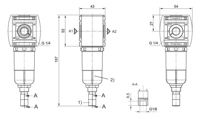
Fully automatic condensate drain
