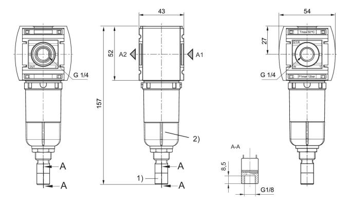
Fully automatic condensate drain
