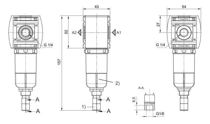
Fully automatic condensate drain
