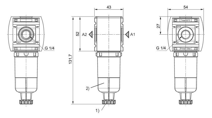
1) Semi-automatic condensate drain 2) Reservoir: polycarbonate
