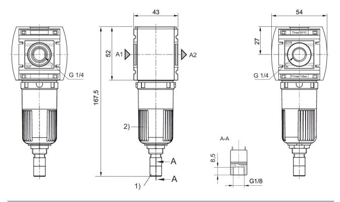
Fully automatic condensate drain
