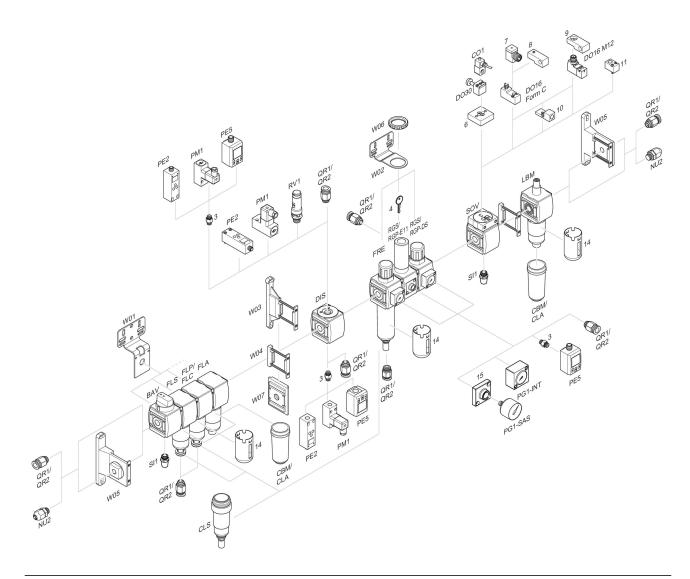
3 = Double nipple 4 = Key for E11 locking 6 = Transition plate DO30 7 = Adapter, Series CON-VP 8 = Mounting aid DO16, form C 9 = Mounting aid DO16, M12 10 = Adapter for external pilot air 11 = Adapter pneumatic operation 14 = Protective guard 15 = Transition plate for assembling a pressure gauge with connection thread G 1/8
