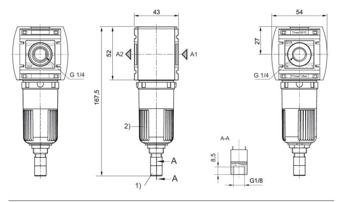
1) Fully automatic condensate drain 2) Reservoir: polycarbonate
