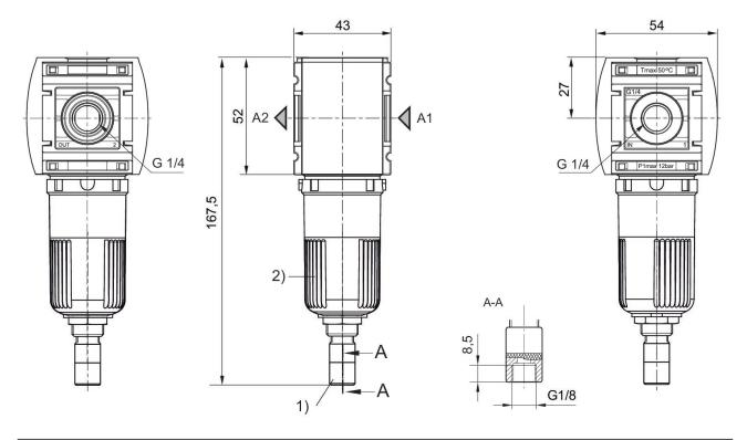
Fully automatic condensate drain
