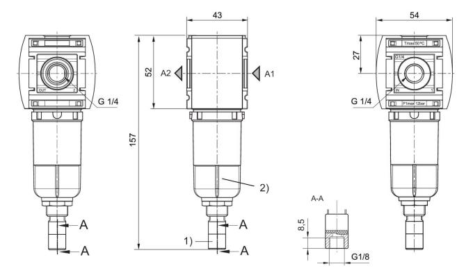
Fully automatic condensate drain
