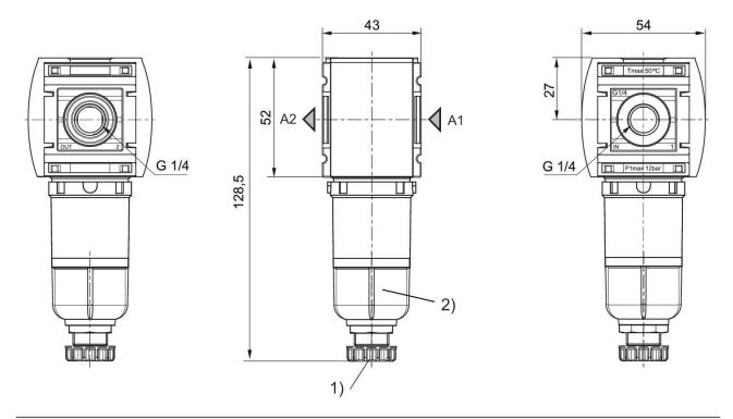
1) Semi-automatic condensate drain 2) Reservoir: metal
