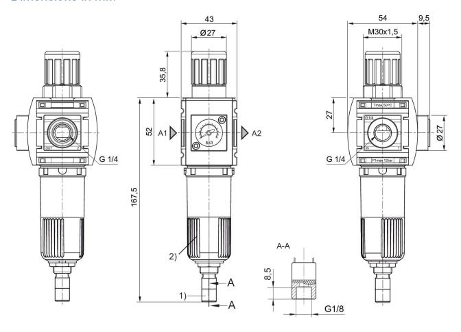
Fully automatic condensate drain
