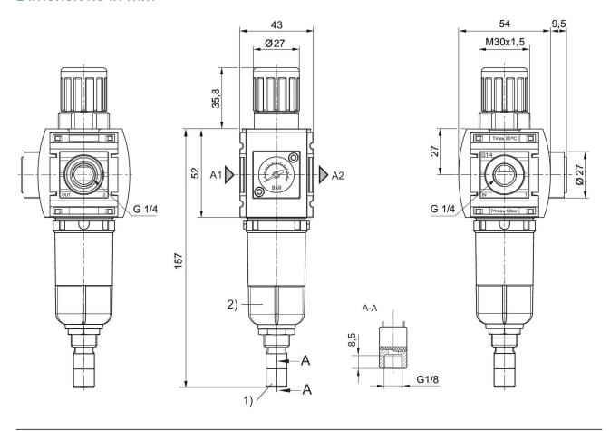
Fully automatic condensate drain
