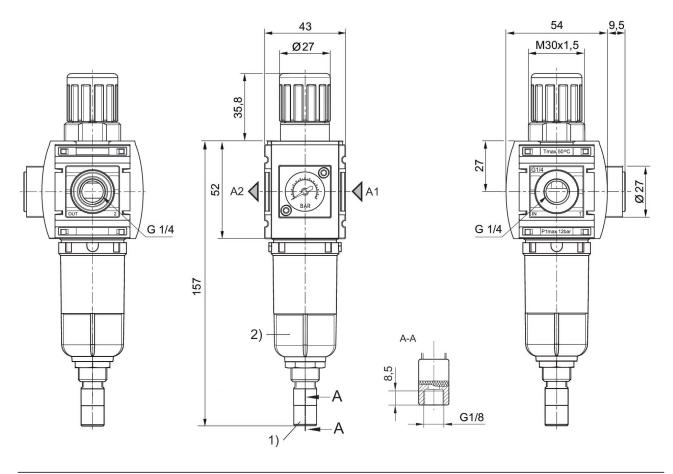
A1 = input A2 = output 1) Fully automatic condensate drain 2) Reservoir: metal
