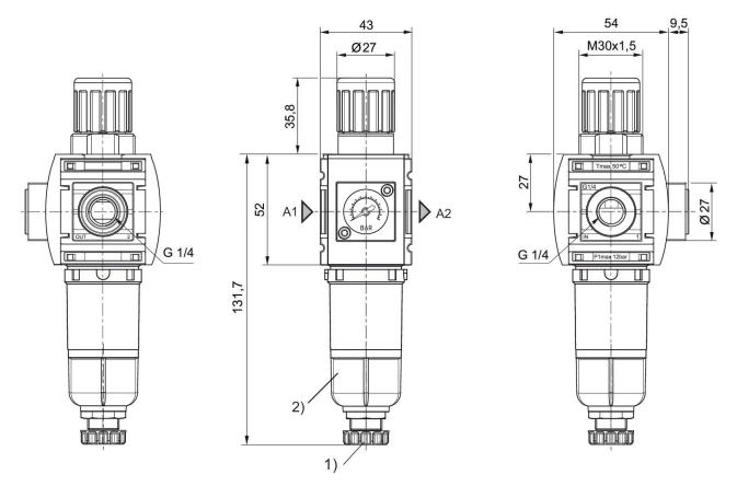
1) Semi-automatic condensate drain 2) Reservoir: metal
