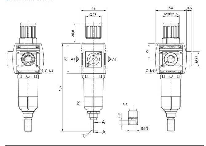
Fully automatic condensate drain
