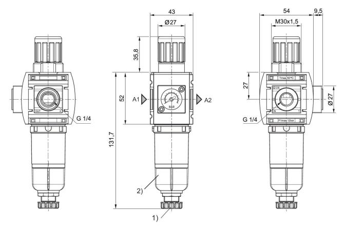
1) Semi-automatic condensate drain 2) Reservoir: metal
