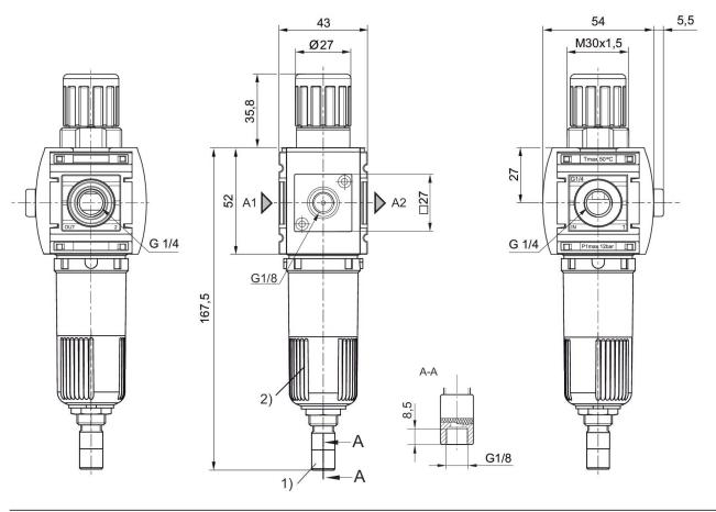
Fully automatic condensate drain
