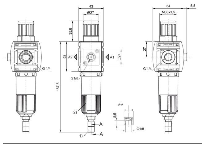
Fully automatic condensate drain
