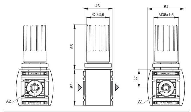
A1 = input A2 = output Panel nut included in scope of delivery
