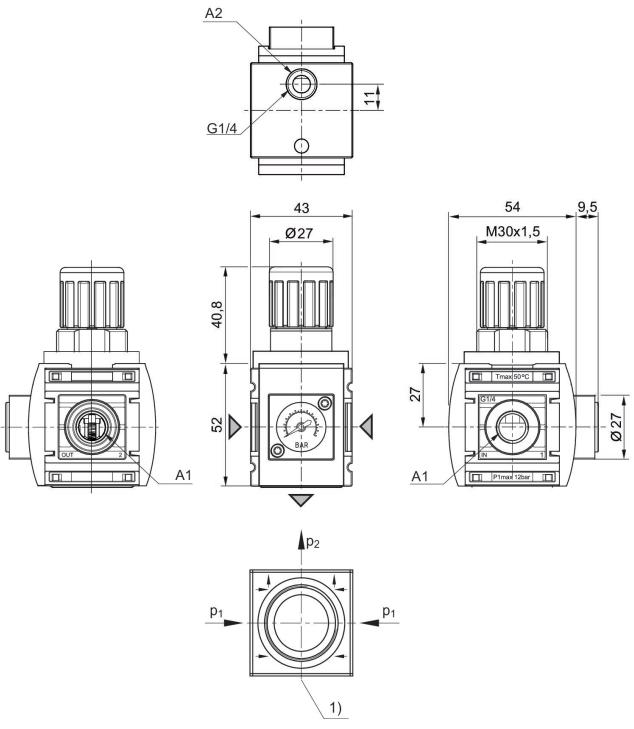
A1 = input A2 = output 1) Pressure gauge connection
