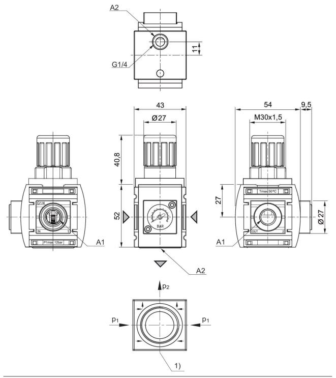
A1 = input A2 = output 1) Pressure gauge connection
