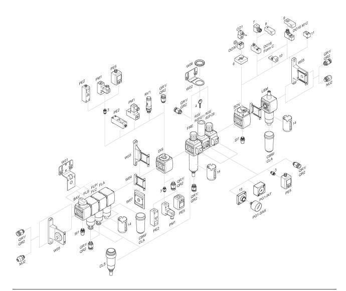
3 = Double nipple 4 = Key for E11 locking 6 = Transition plate DO30 7 = Adapter, Series CON-VP 8 = Mounting aid DO16, form C 9 = Mounting aid DO16, M12 10 = Adapter for external pilot air 11 = Adapter pneumatic operation 14 = Protective guard 15 = Transition plate for assembling a pressure gauge with connection thread G 1/8
