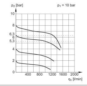
p1 = Working pressure p2 = Secondary pressure
