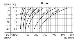
DTP-E: pressure dew point input, DTP-A: pressure dew point output, Qv: input flow rate (output flow rate + purge air).
