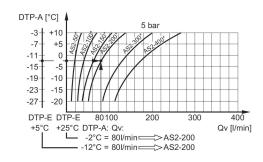
Result: membrane dryer series AS2-200 (with a Qn of 200 l/min), part no. R412006081
