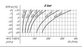
DTP-E: pressure dew point input, DTP-A: pressure dew point output, Qv: input flow rate (output flow rate + purge air). \* Nominal flow Qn
