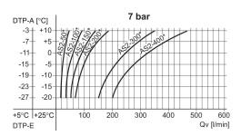
DTP-E: pressure dew point input, DTP-A: pressure dew point output, Qv: input flow rate (output flow rate + purge air).
