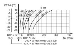
Result: membrane dryer series AS2-200 (with a Qn of 200 l/min), part no. R412006081
