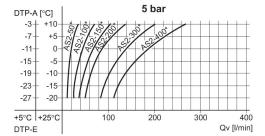
DTP-E: pressure dew point input, DTP-A: pressure dew point output, Qv: input flow rate (output flow rate + purge air).
