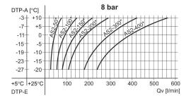
$\label{eq:decomposition} \mbox{DTP-E: pressure dew point input, DTP-A: pressure dew point output, Qv:}$ input flow rate (output flow rate + purge air).
