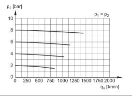
p1 = Working pressure p2 = Secondary pressure qn = Nominal flow
