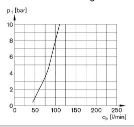
p1 = Working pressure qn = Nominal flow Flow rate characteristic, p2 = 0,05 - 7 bar
