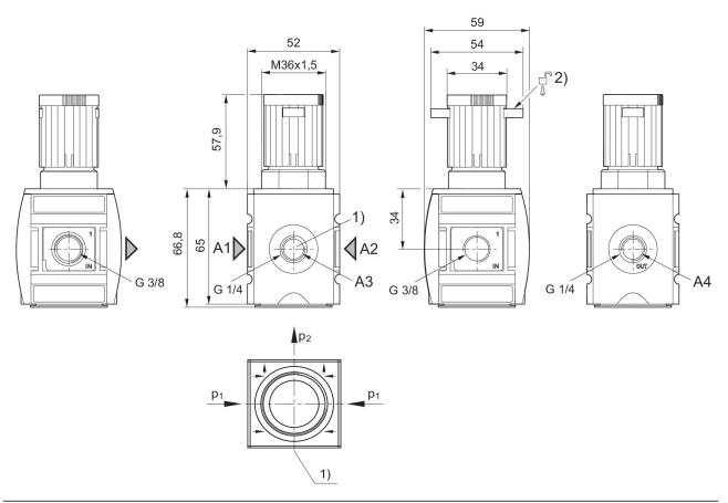
A1 = input A2 = output A3 = pressure gauge connection A4 = output 1) Pressure gauge connection 2) Mounting option for padlocks, max. shackle Ø 8
