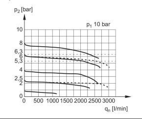
p1 = Working pressure p2 = Secondary pressure qn = Nominal flow
