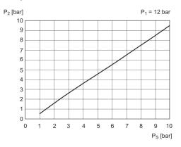
p1 = Working pressure p2 = Secondary pressure PS = control pressure
