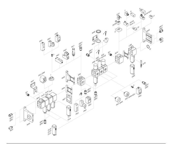
1 = contamination display 3 = Double nipple 4 = Key for E11 locking 5 = mortise lock 6 = Transition plate DO30 7 = Adapter, Series CON-VP 8 = Mounting aid DO16, form C 9 = Mounting aid DO16, M12 10 = Adapter for external pilot air 11 = Adapter pneumatic operation 12 = Sealing ring
