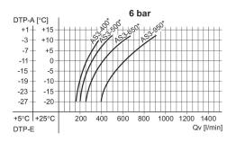
DTP-E: pressure dew point input, DTP-A: pressure dew point output, Qv: input flow rate (output flow rate + purge air).
