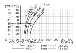
Result: membrane dryer series AS3-950 (with a Qn of 950 l/min), part no. R412007081
