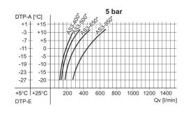
DTP-E: pressure dew point input, DTP-A: pressure dew point output, Qv: input flow rate (output flow rate + purge air). \* Nominal flow On
