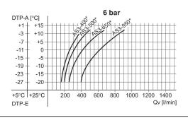
DTP-E: pressure dew point input, DTP-A: pressure dew point output, Qv: input flow rate (output flow rate + purge air). \* Nominal flow Qn
