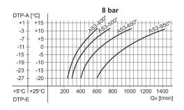
DTP-E: pressure dew point input, DTP-A: pressure dew point output, Qv: input flow rate (output flow rate + purge air). \* Nominal flow Qn
