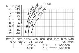
Result: membrane dryer series AS3-950 (with a Qn of 950 l/min), part no. R412007081 \* Nominal flow Qn
