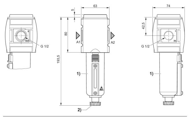
A1 = input A2 = output 1) Plastic reservoir and protective guard with window 2) Semi-automatic condensate drain
