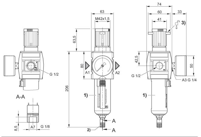
A1 = input A2 = output A3 = pressure gauge connection A7 = condensate drain
