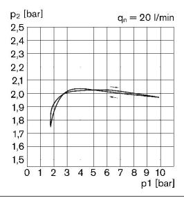
p1 = Working pressure p2 = Secondary pressure qn = Nominal flow
