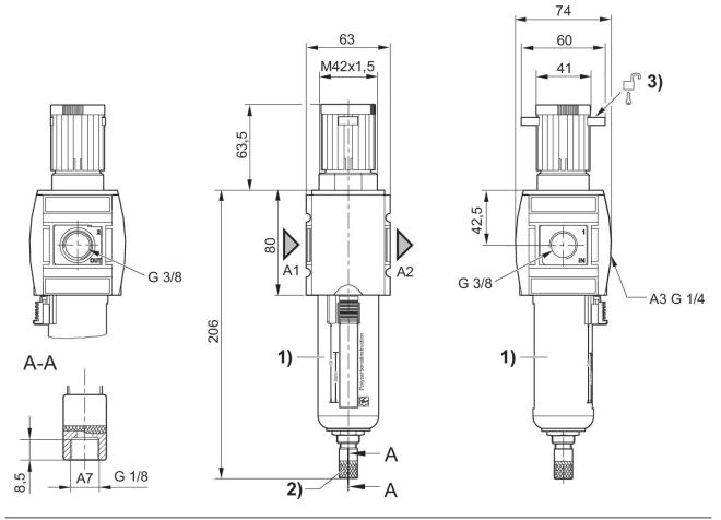
A1 = input A2 = output A3 = pressure gauge connection A7 = condensate drain
