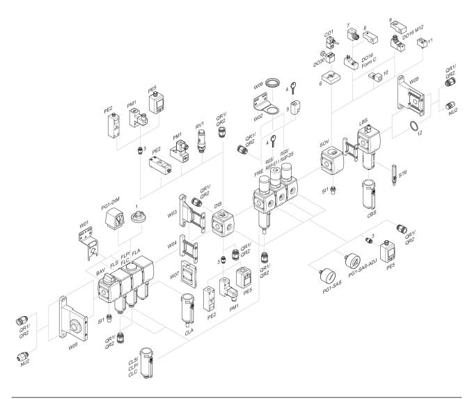
1 = contamination display 3 = Double nipple 4 = Key for E11 locking 5 = mortise lock 6 = Transition plate DO30 7 = Adapter, Series CON-VP 8 = Mounting aid DO16, form C 9 = Mounting aid DO16, M12 10 = Adapter for external pilot air 11 = Adapter pneumatic operation 12 = Sealing ring
