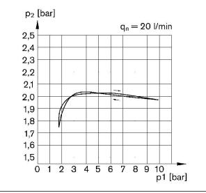
p1 = Working pressure p2 = Secondary pressure
