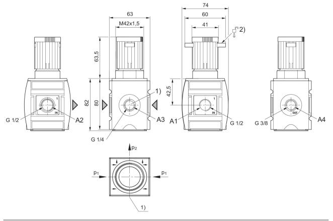
A1 = input A2 = output A3 = pressure gauge connection A4 = controlled connection
