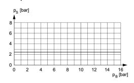
minimum pilot pressure depending on working pressure
