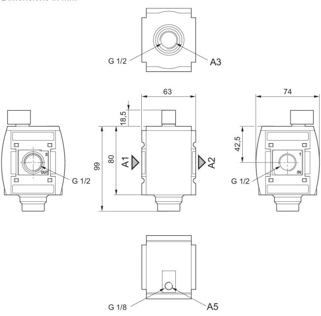
A1 = input A2 = output A3 = ventilation port A5 = Control pressure connection
