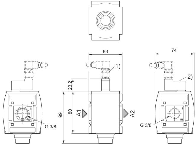
A1 = input A2 = output 1) plug M12
