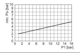
p1 = Working pressure PS = control pressure
